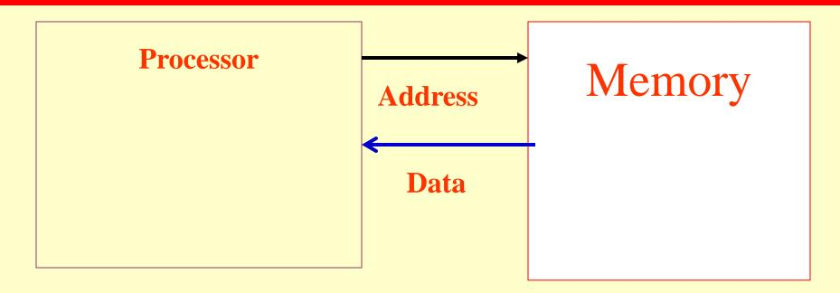
Step 1) Processor requests instruction from memory using address in Program Counter PC register
